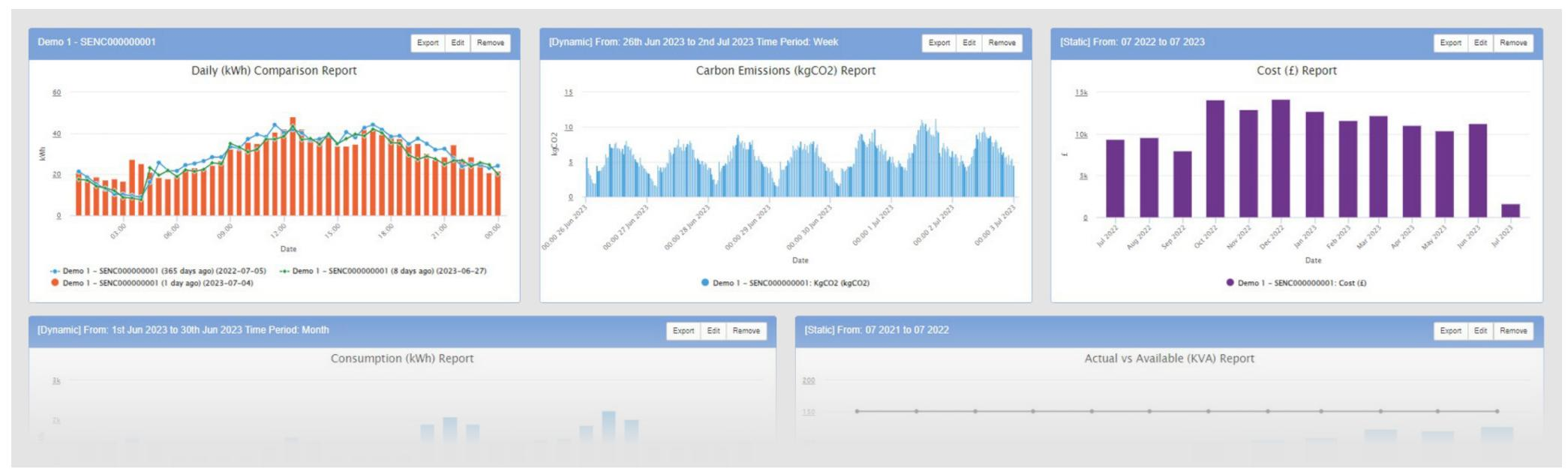
Daily (kWh) Comparison Report - Consumption (kWh) - This report displays half hourly kilowatt hour (kWh) data from your meter. The orange bars indicate consumption for a day, the green line indicates consumption for the same period in the previous week and the blue line indicates consumption for the same period in the previous year.
